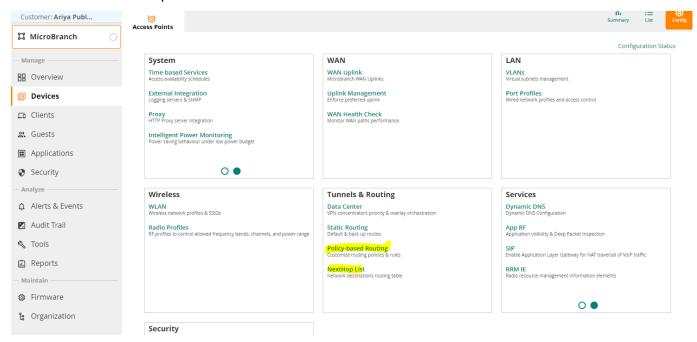
First we'll add all the IPSEC tunnels to the NextHop list so we can then use it in our PBR. NextHop list makes it easier for cases where you have 2 or more IPSEC tunnels that we can forward traffic. In our case we have 2x IPSEC tunnels for each of the uplinks (eth0 and LTE). Note that highest priority is given to Aruba SSE primary IPSEC tunnel through Eth0 uplink followed by Aruba SSE secondary IPSEC tunnel and so on.
