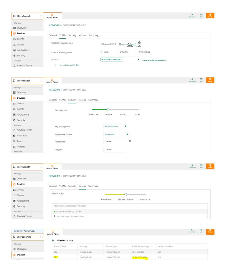
Now we need a mechanism to selectively redirect user's HTTP/HTTPS traffic to Aruba SSE, for inspection and policy compliance. These are the users that will be connecting to RL3 wlan. We'll use Policy Base Routing (PBR) for it.
