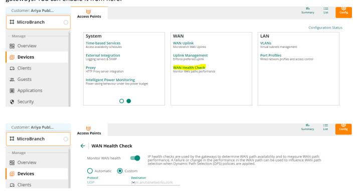
Once you enable "Monitor WAN Health", the probes are sent through the underlay and based on the probe response the uplinks are marked as available or not. The probes are sent 5x UDP or ICMP every 10 sec. When a probe is lost then the frequency of sending probes increases to every 2 sec. The details are mentioned <a href="here">here</a>.
