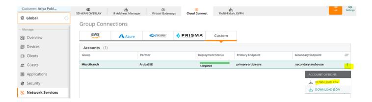
You need to open the CSV file and the information that we need are "Source Identity" and PSKs that corresponds to your microbranch APs. You need to copy it. Take particular note of the uplink name as the Identity and PSKs are specific to the uplinks. We'll use these when we configure Aruba SSE to allow these IPSEC tunnels.
