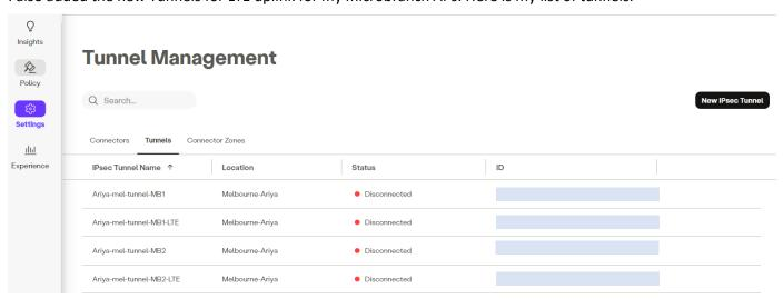
I have 2x MB APs and each have 2 uplinks (E0 and LTE), that is why I need 4x tunnels to be configured in Aruba SSE dashboard. Once you configure the tunnels here, then its matter of time for the IPSEC tunnels to be established. I have connected my microbranch2 AP. Note that all of them are associated with location = "Melbourne-Ariya-MB".
