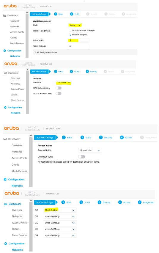
Once you have configured this profile and assigned it to 0/0 as shown above, you can then connect the LAN switch to this Eth0 interface of the Mesh point AP.
