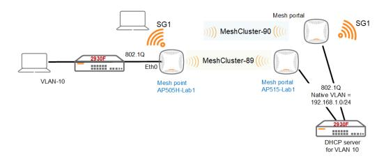
Note that we already have configured the mesh cluster "MeshCluster-89", we'll continue with the Instant cluster level configuration of "MeshCluster-90". The only command needed is this.
