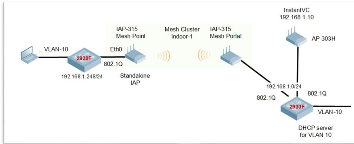
The laptop (with the MAC address of F0:DE:F1:64:0A:82) gets an IP address from VLAN 10 at the far side.
