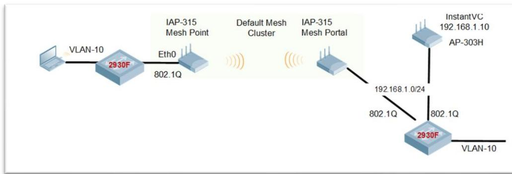
The second one is showing the configuration steps involved in setting manual mesh cluster for a specific Mesh porta/point with EO bridging.
