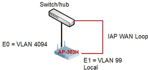
We should check the port status and see that loop-protect is on for E1. And both E0 and E1 are up.
