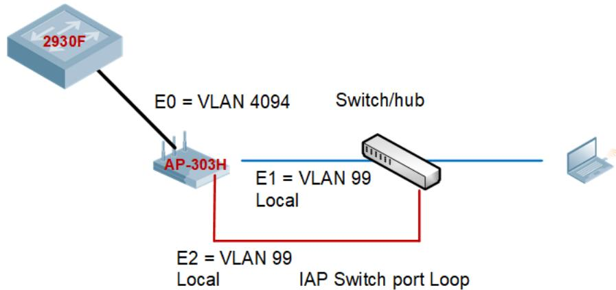
First we should enable loop protect on E2 port
